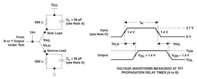
A-TO-B LOAD OR A-TO-Y LOAD (Totem Pole)
